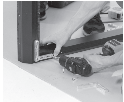
IV.15. Attach lower horizontal profiles along the way.
